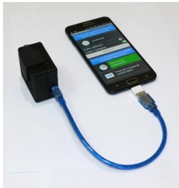
Fig. 6: An integrated sensor assembly for fluoride sensing.
